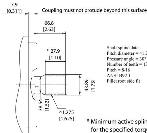
\* Minimum active spline length for the specified torque ratings
