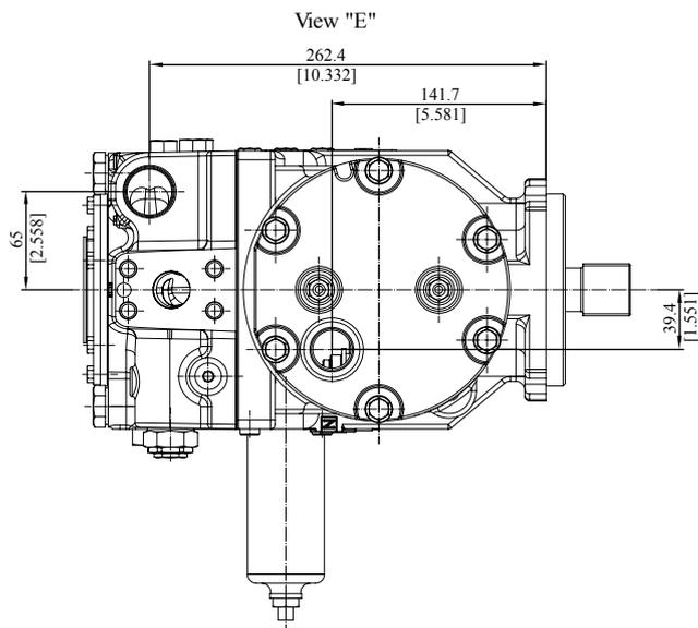
*Integrated NFPE control, endcap twin ports*
