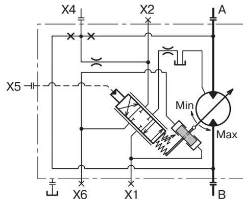
HP S 01 E schematic(pool in a balanced, mid-pos.)
