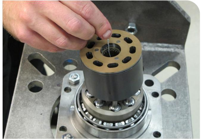
49. Make sure the support pin is in correct position by using a steel wire.
