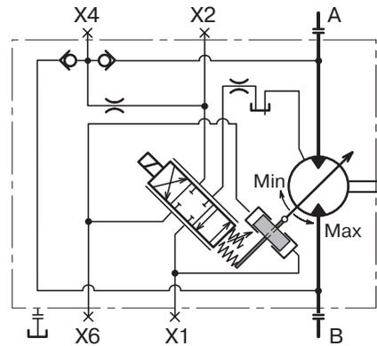
EPH 01 I schematic (spool in balanced, mid-pos.)
