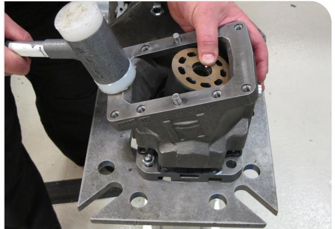
51. Assemble the bearing housing. Carefully knock it down with a plastic hammer. Secure the housing by assembling one screw.
