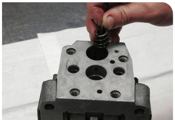
30. Assemble the threshold spring.
