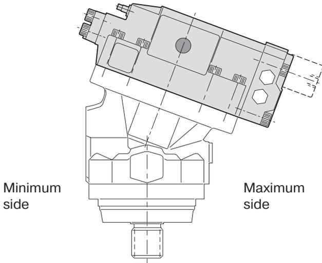
AC and AH control should be assembled with the control cover at the maximum side.
