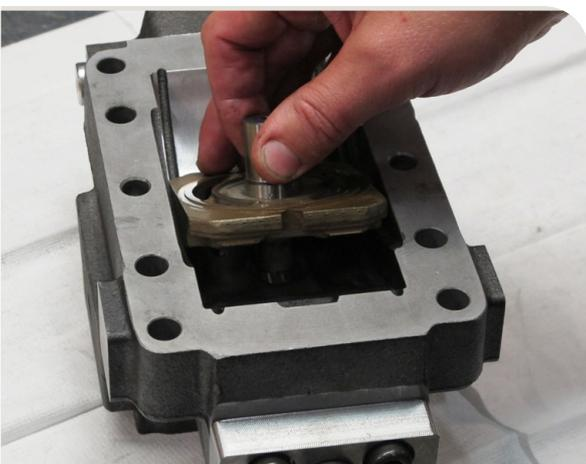
41. Assemble the valve segment in the end cap. The slot in the valve segment against the cover side.
