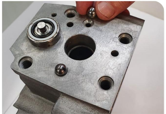
35. Assemble the check valve balls.
