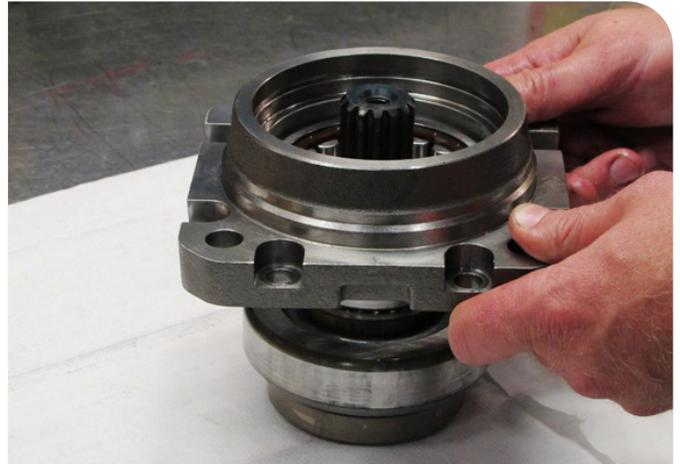
2. Press down the roller bearing with the text upwards into the flange and assemble it on the shaft package.
