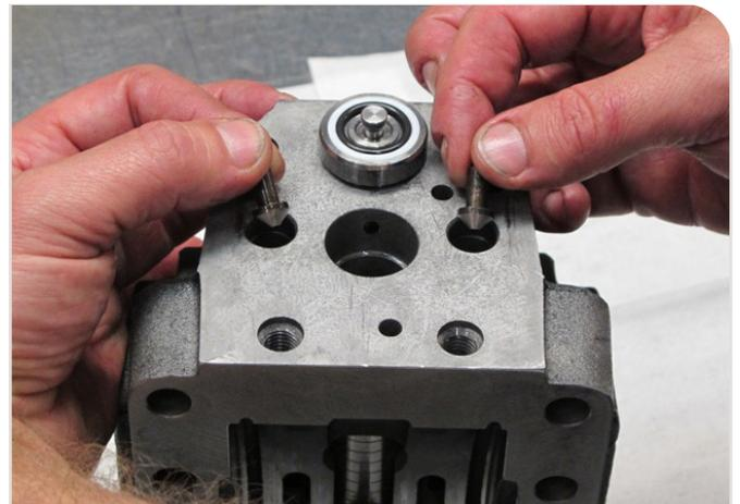
34. Assemble the valve cones.
