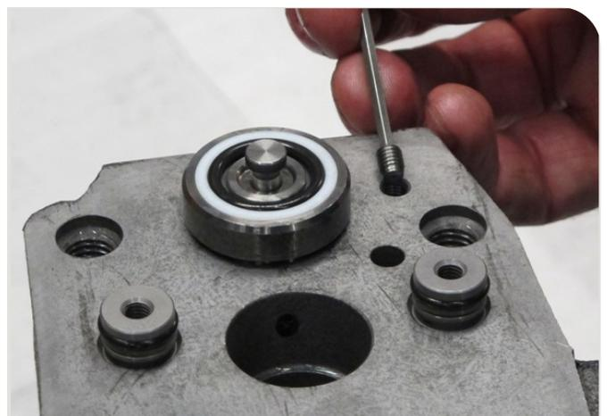
36. Assemble the nozzles and torque them to  $1,2 \pm 0,2$  Nm.
