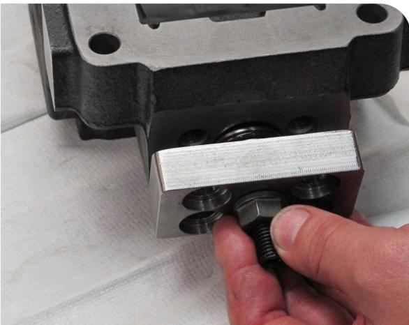
39. Assemble the cover assy. Make sure not to damage the O-ring.
