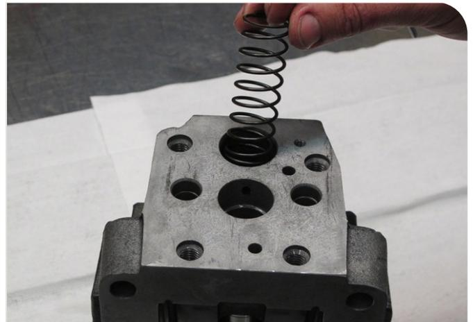
28. Assemble the modulating spring.
