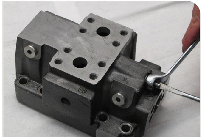
20. Assemble the adjusting screw and seal nut.
