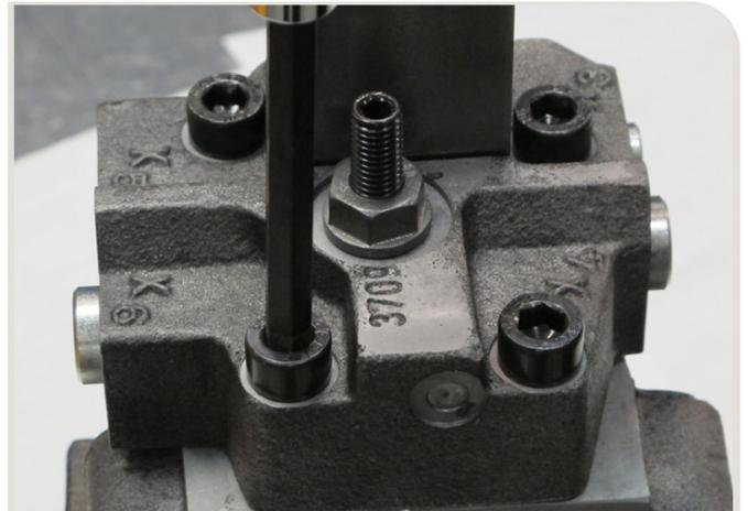
38. Torque the screws to  $65\pm 10$  Nm for V12-60 – -110,  $105\pm 20$  Nm for V12-160.
