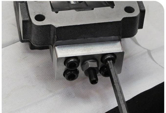
40. Torque the screws to  $65 \pm 10$  Nm for V12-60 – -110,  $105 \pm 20$  Nm for V12-160.
