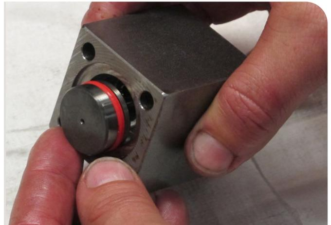
14. Assemble the control piston in the AH-housing.
