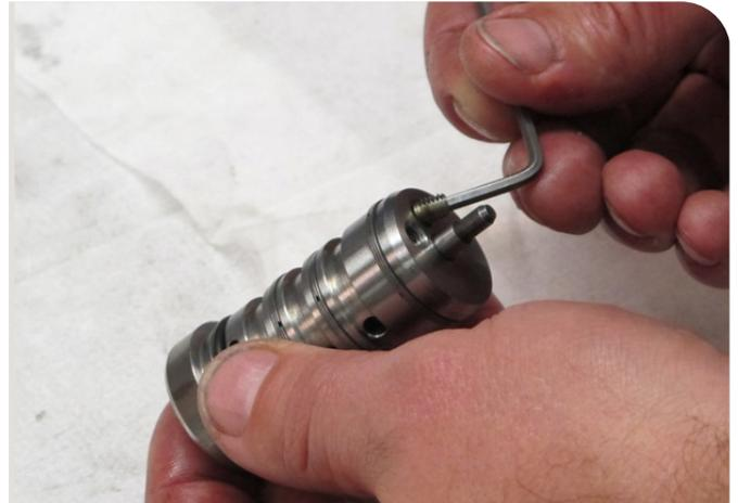
32. Assemble the nozzles and torque them to  $1,2 \pm 0,2$  Nm.
