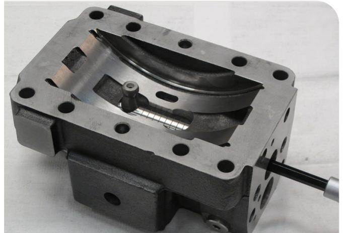
26. Torque the set screw to  $26 \pm 6$  Nm. Move the companion pin back and forward to make sure it moves smooth.
