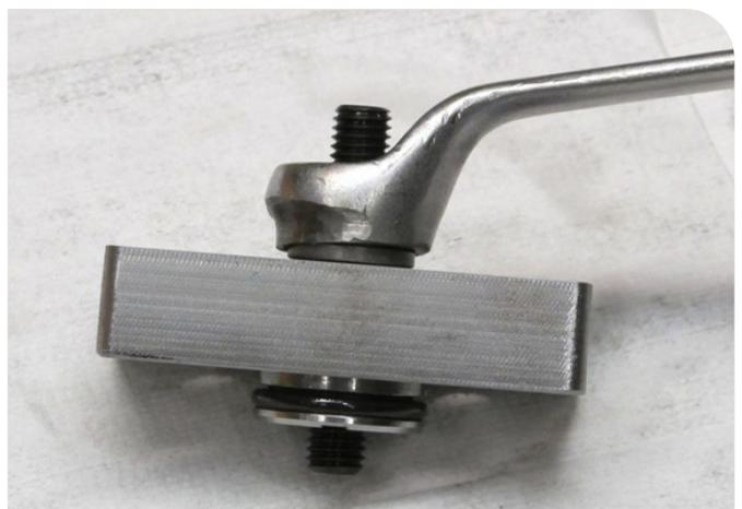
12. Assemble the displacement setting screw, seal nut and the O-ring.
