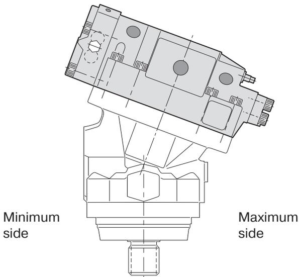
HO and HP control should be assembled with the control cover at the minimum side.
