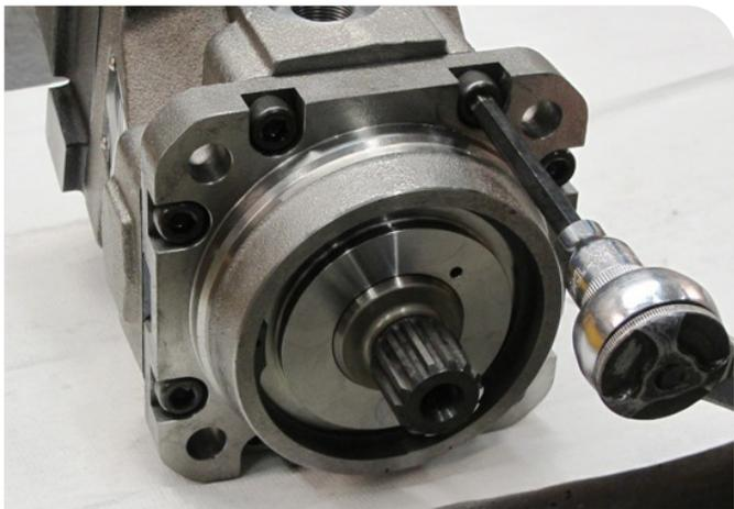
55. Assemble the screws and torque the screws to  $65\pm 10$  Nm for V12-60/80 and  $105\pm 20$  Nm for V12-110/160.
