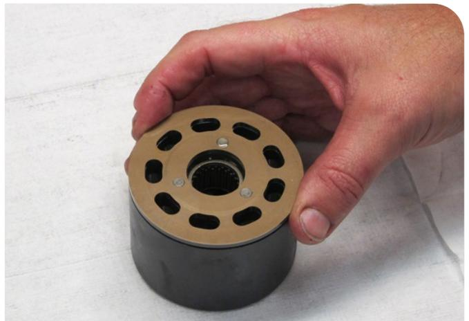
10. Assemble the sliding plate.
