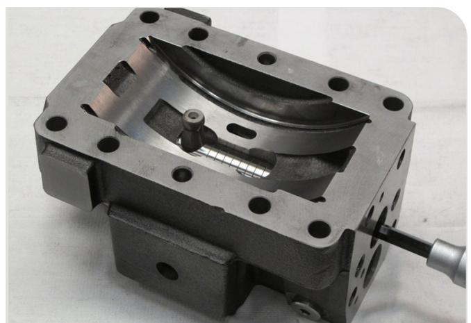
24. Torque the set screw to 14±4 Nm.
