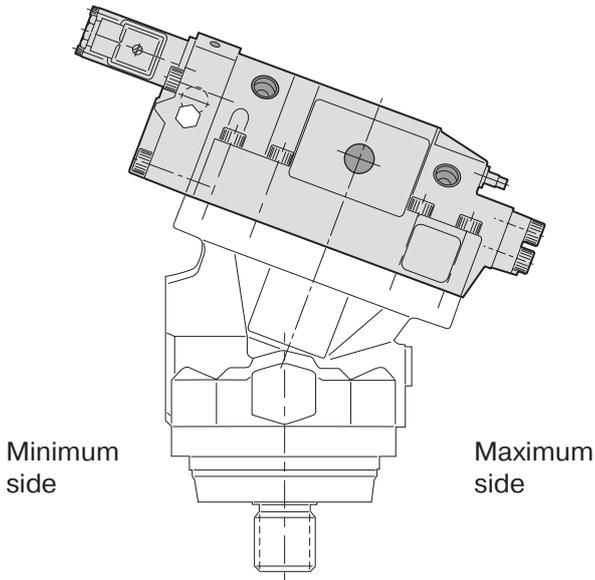
EO and EP control should be assembled with the control cover at the minimum side.
