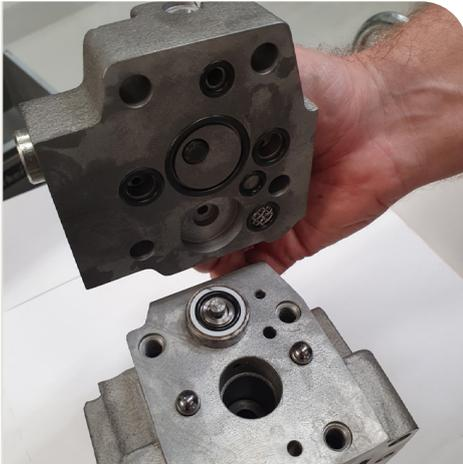
37. Assemble the control cover assy. Make sure the O-rings and check valve balls are in correct position.
