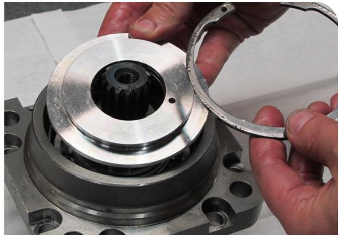
8. Assemble the seal carrier with shaft seal and the retaining ring. Make sure it is all the way into the groove.
