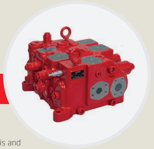
**The KLW** is a flow-sharing, load-sensing main control valve specifically designed for wheel loaders. It provides low hysteresis and superior pressure-drop characteristics to deliver high performance and excellent levels of efficiency.
