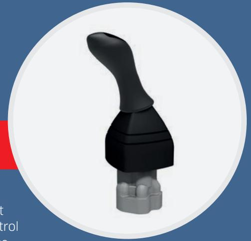
Our PV series valves are pressure-reducing type pilot valves that allow operators to simultaneously control spools of multiple control valves as well as the tilting angle of variable displacement pumps. The operational torque can be reduced to meet your requirements (Patent registered), while the small operational force enables minute control, reduced pressure drop and quick response.
