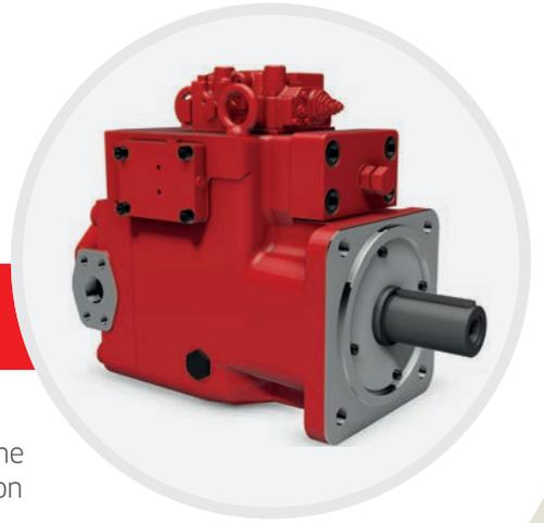
The K7VG series of high-pressure swash plate type pumps was developed for general industrial machinery use. The adoption of the high-load bearings and friction-free contacting mechanism of piston shoes, results in a high level of reliability and long life.
