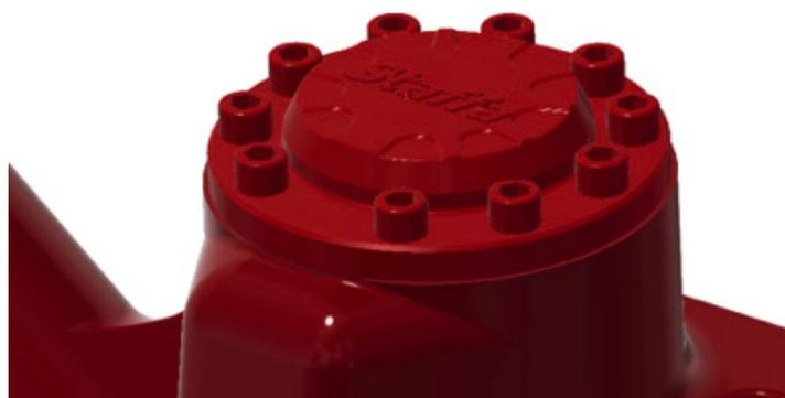
When top-coat paint solutions are applied to any surface, the coverage can easily become sub-optimal for very complex shapes. As the protection of the Staffa motor's external surfaces is critical in corrosive environments, the marine-style cylinder head, which is geometrically simplified in comparison to the standard design, can be specified for all HMF motors to aid in the optimal application of the top-coat paint solution.
