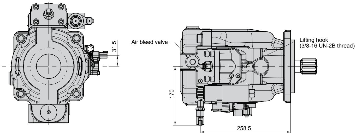
**Port option D** (pump with metric threads)
