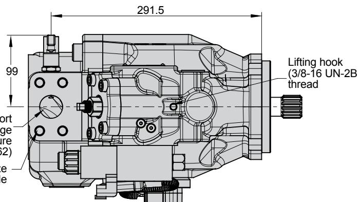
**Port option D** (pump with metric threads)
