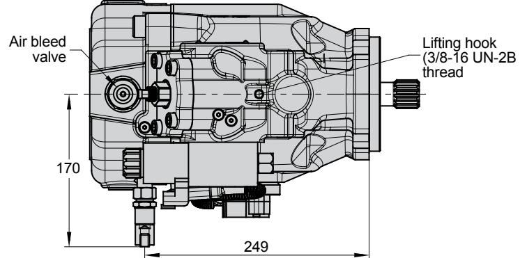
**Port option D** (pump with metric threads)
