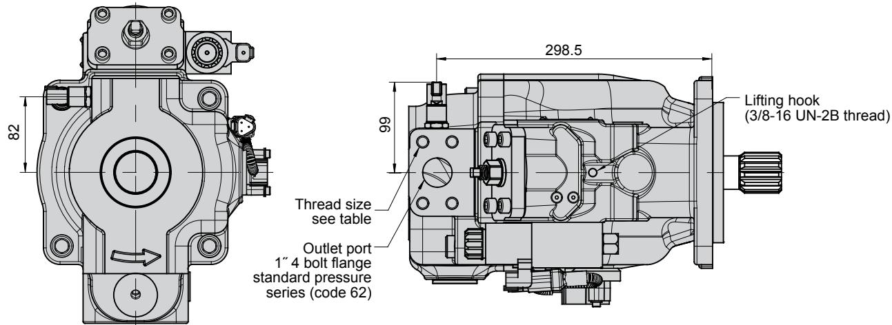
**Port option D** (pump with metric threads)
